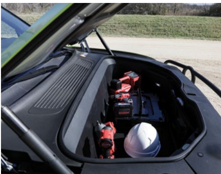
Frunk: A sealed, lockable compartment for tools and safety gear, protected from the elements
