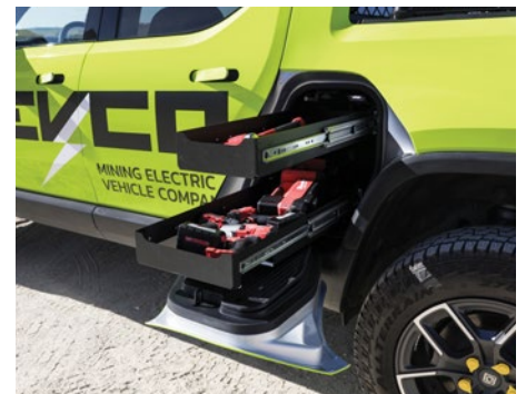
Gear Tunnel: A tunnel between the cab and bed for longer items like shovels or custom drawers
